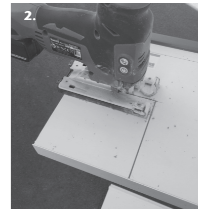
2. Use a jig saw to cut the notch out
