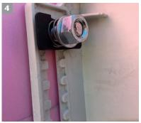
Screw the nut off. Slide the light shaft with the grating in place onto the heavy-duty anchors. Set the locking block in place, slide the spring and washer over, slightly tighten the nut.
