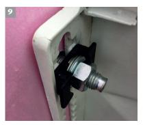
After final height adjustment, tighten the nut.
